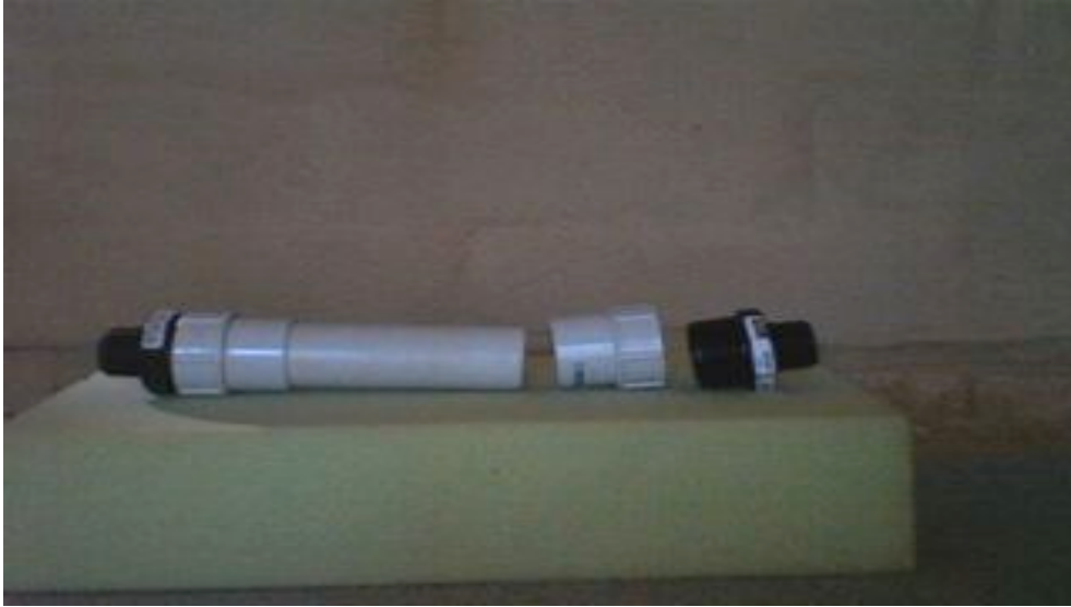
Creek washer with one end glued. Leave the other end unglued.
