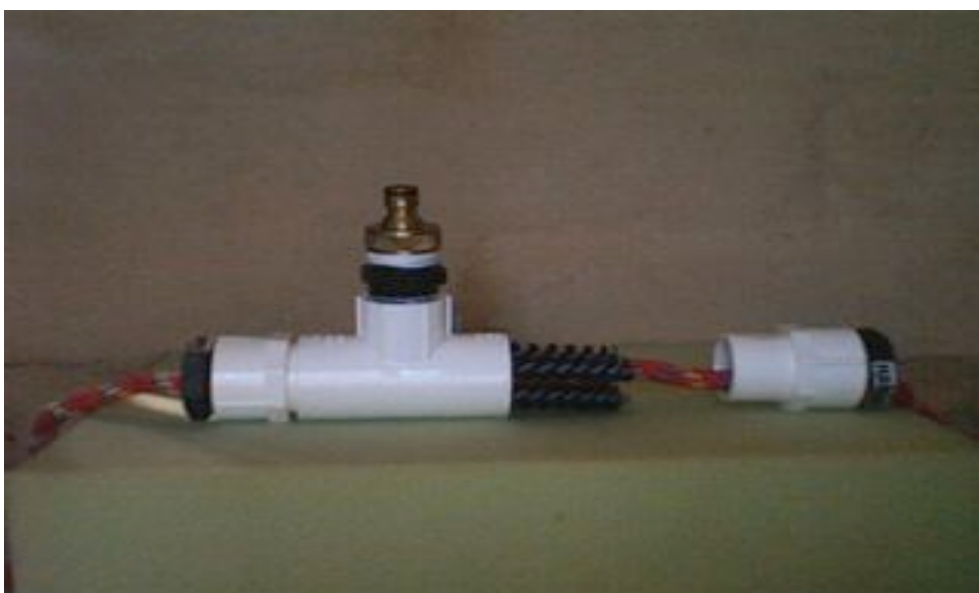
The hose washer with ONE end glued and the other ready to be assembled and which is NEVER glued.
